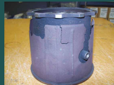
P/N# 1-140-590-07 as removed from engine (low carbon steel)
