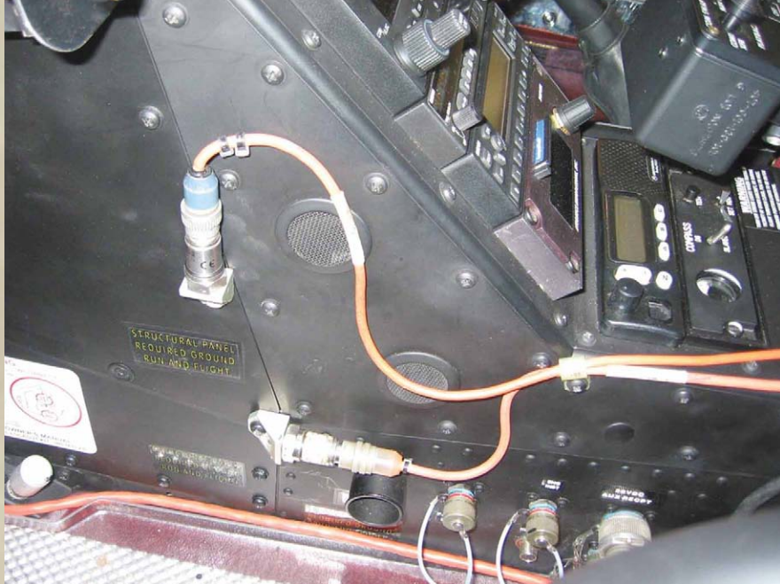
Correct cable/accelerometer installation
