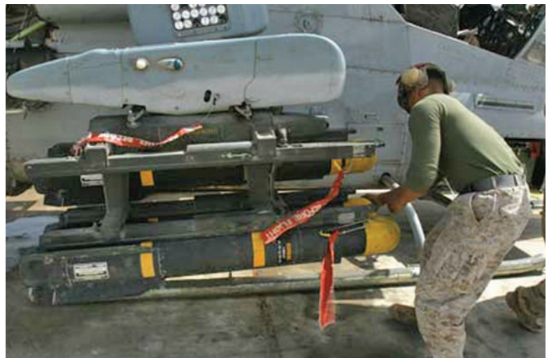
Right: Vogen loads an AGM-114 Hellfire missile aboard an AH-1W Super Cobra helicopter at Al Taqaddum, Iraq, March 25.
