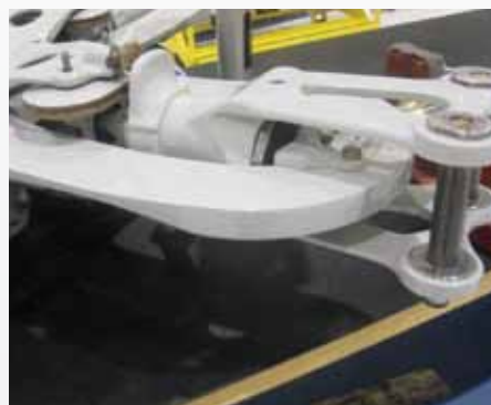
Figure 2. Feathering bearing installed in hub assembly
