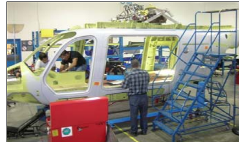
The cabin of 429 aircraft No. 1 is shown in final assembly at the Mirabel manufacturing facility. The cabin, nose and aft fuselage were mated in early July.
