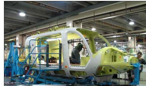
The cabin of 429 aircraft No. 2 is assembled at the Mirabel manufacturing facility.
